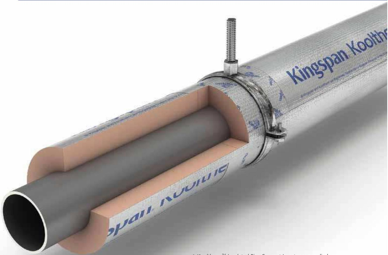
\* Kooltherm™ Insulated Pipe Support Inserts are supplied with a self-adhesive lap. Kooltherm™ Pipe Insulation sections should be vapour sealed to the pipe support.
